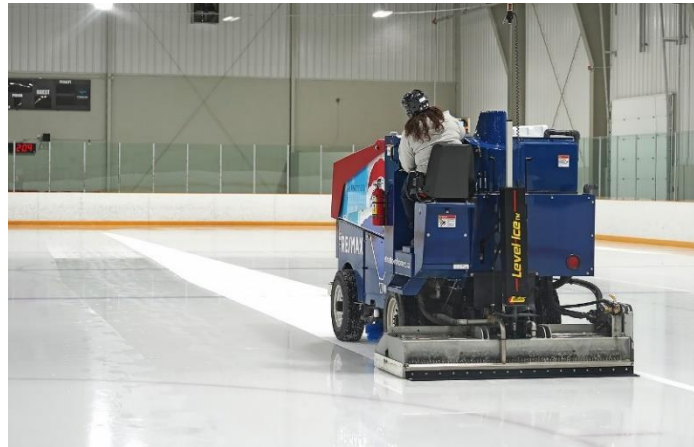
Figure 5 Electric ice resurfacer in use
